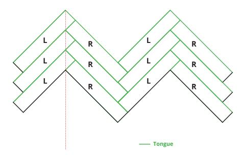
After the first line has been completed, you can start with installation of the lines next to the first line, creating the "W" shape from the herringbone.
