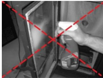
Figure 39 – Incorrect cleaning of the glass
