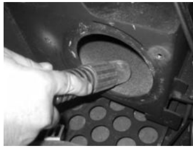
Figure 38 – Vacuum the air flow pipes
