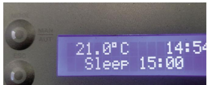
The display will then switch between the normal screen and a screen similar to above showing the current time and the sleep time at which the stove will switch off.
