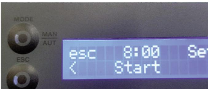
To set the starting time for Programme P1, press "set". The display starts to flash. Press the "+" or "-" key to select the time and then press "ok" to confirm. Press the "+" key to go to the P1 "Stop" menu.
