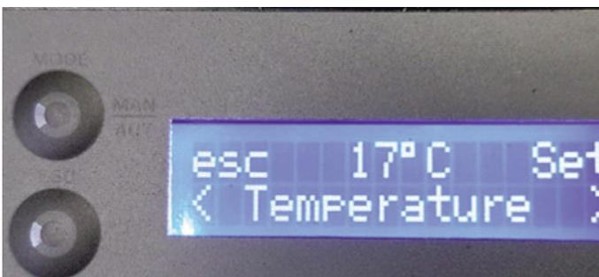
To set the set point temperature for Programme P1, press "Set". The display starts to flash. Press the "+" or "-" key to select the desired temperature, followed by "Ok" to confirm.
