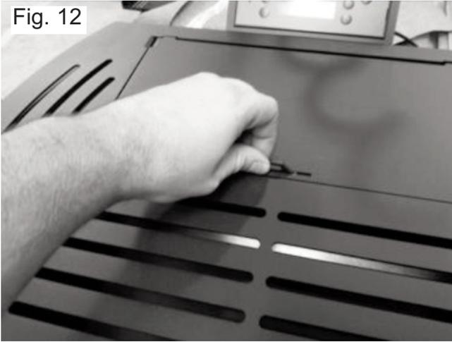
The reservoir will hold approx 11 kg, to fill the hopper carefully cut the corner of the bag so the pellets can be poured into the hopper without spilling outside of the rubber seal. Do not pour dust into the hopper as it can impair the feed screw mechanism.
