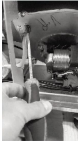
To remove the fan motor and impeller assembly specialist tools will be required to access the least accessible screw. See picture of suitable tool including pz1 screw tip.
