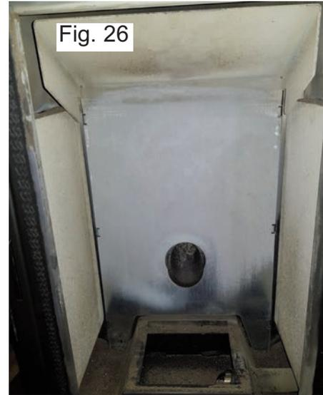
To remove the vermiculite lift it with one hand and the baffle with the other, when both are raised move the vermiculite out over the tab at the bottom edge allowing the vermiculite then be removed. Then remove the flue baffle.
