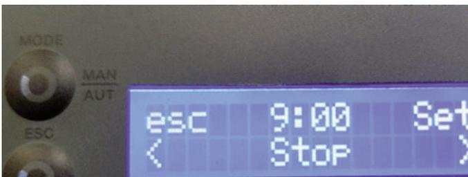
To set the stopping time for Programme P1, press "set". The display starts to flash. Press the "+" or "-" key to select the time and then press "ok" to confirm. Press the "+" key to go to the "Air Temperature" menu.
