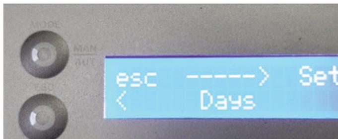
To select the days of the week that you want P1 Programme to run, press "set" and then select the day of the week using the "-" and "+" keys. Press "set". The display starts to flash. Select "On" or "Off" using the "-" and "+" keys. Press "ok" to confirm the selection. Press the "esc" key to go to the "Days" menu. Press the "esc" key again to go to the "program" menu. Press the "+" key to move on to the next menu.
